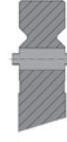
HD Safety-Pin Applicable for tool weight > 12.5 kg/28 lbs - < 150 kg/331 lbs. (NS I + II)
